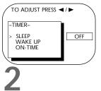
Press the PLAY/▲ button or the STOP/▼ button to select SLEEP. Then press the REW(ind)/◀ button or the F.FWD/▶ button to select 30 MIN(utes), 60 MIN(utes), 90 MIN(utes), 120 MIN(utes) or OFF. (You can not set the sleep timer during a recording.)
